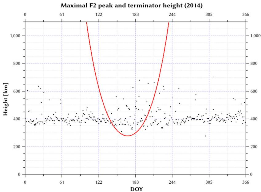
Fig. 7. The daily maximal height of the  $F_2$  peak (black dots) and the boundary of the permanent sunlight (red line) during 2014. (For interpretation of the references to color in this figure legend, the reader is referred to the web version of this article.)
