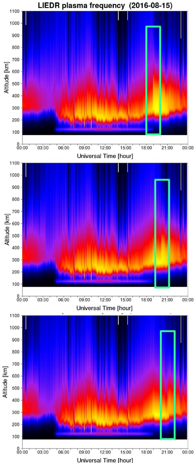
Fig. 9. Plasma frequency representation of the LIEDR output calculated for 15 August 2016 using the measurements from Dourbes. The top-panel was produced switching between day-time and night-time profiles based on the times of sunrise and sunset at sea-level, the middle panel using the times at a fixed 100 km altitude, and the bottom panel using the times at the  $F_2$  peak altitude. An artificial discontinuity in the profiograms happening around sunset is marked by a rectangle.
