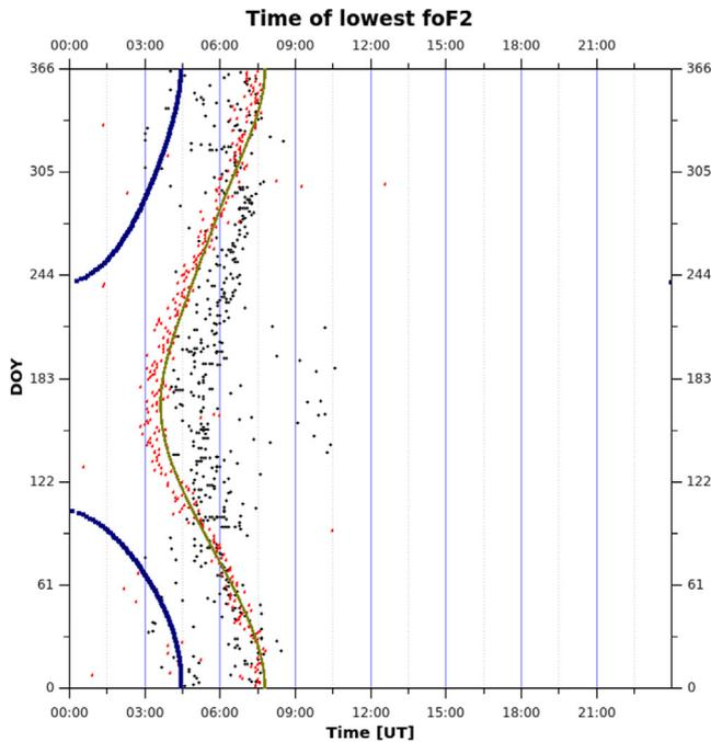
Fig. 8. The times of the daily minima for the critical frequency  $f_oF_2$  (blue dots) and the first appearances of the  $E$  layer (red dots) during 2014. The solid lines show the time of sunrise at 90 km (green) and 1100 km (blue). (For interpretation of the references to color in this figure legend, the reader is referred to the web version of this article.)
