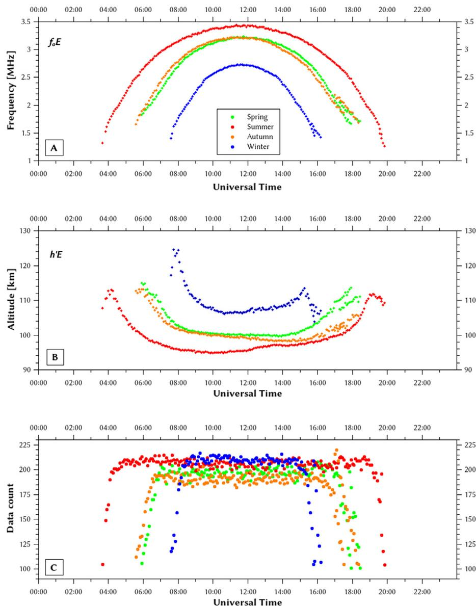
Fig. 5. Average diurnal behaviour of the  $E$ -layer critical frequency  $f_oE$  (panel A) and (virtual) height  $h'E$  (panel B) at different seasons as measured by the Dourbes digisonde. Panel (C): Number of days during which an  $E$  layer was detected from ionosonde measurements (5-min cadence) at Dourbes at the times of the soundings, plotted separately for each of the four seasons.
