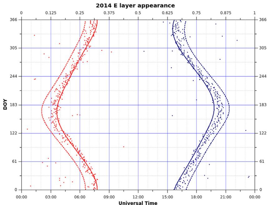
Fig. 4. The times of the first (red dots) and last (blue dots) detections of the E layer above Dourbes for each day of year 2014, approximated at sea level (solid curves) and at an altitude of 100 km (dashed curves). (For interpretation of the references to color in this figure legend, the reader is referred to the web version of this article.)
